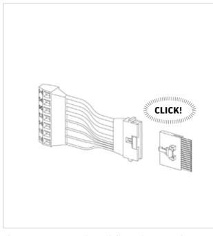
Plug connections must always click into place. Press the latch to unlock.
